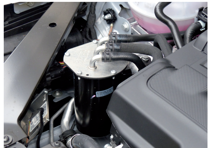
Figure 3: Filter housing in the engine bay
